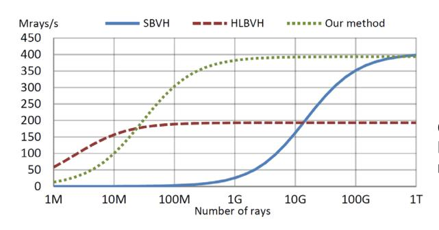
Comparison of different BVH construction methods. From [1].
